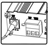
12. The SD-250 can be powered either by the hardwired Euroblock connector, or via barrel connector with the included power supply (shown above). Use a safety approved (UL/ETL, etc...) 32V 3.75A power supply.
