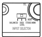
11. Select desired input via input selector switch located on the front of the SD-250.
