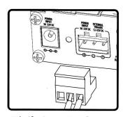
13b. If using external trigger, run the trigger positive wire into "T" and the trigger negative wire into "-" using the 3 pin Euroblock. Note: If using both external trigger and hard wired power, both negative wires will share the "-" Euroblock input.
