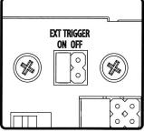
13a. The SD-250 can be turned on and off with an external 12v-32v DC trigger. To enable, move the jumper to "on."
