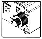
15. Adjust volume with knob on front of amplifier. Inner knob controls left channel and outer knob controls right channel.
