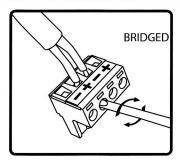
8b. Bridged: connect single pair of speaker wire to the center + and - terminals of 4 pin Euroblock. <u>DO NOT</u> use outside terminals.
