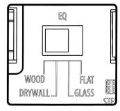
14. The SD-250 provides equalization settings for wood, drywall or glass SolidDrive installations. The EQ may also be set to flat response. Move the slide switch to the desired setting for your installation.
